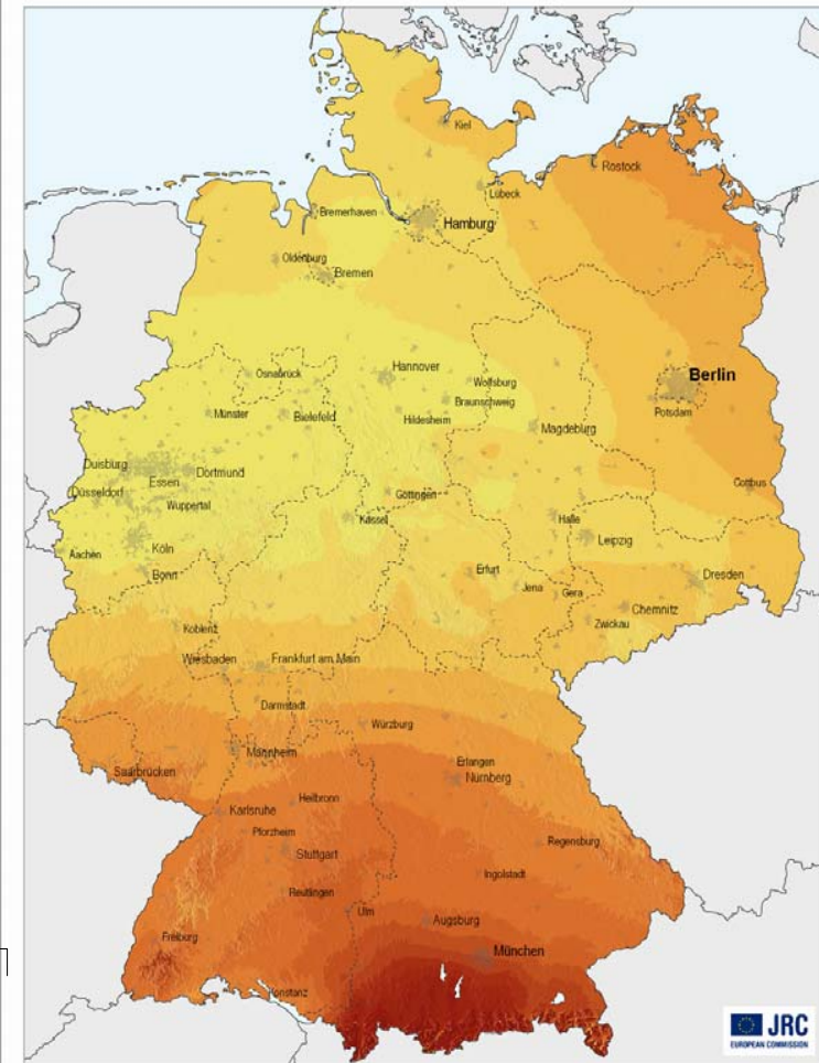
Global irradiation and solar electricity potential Optimally-inclined photovoltaic modules
