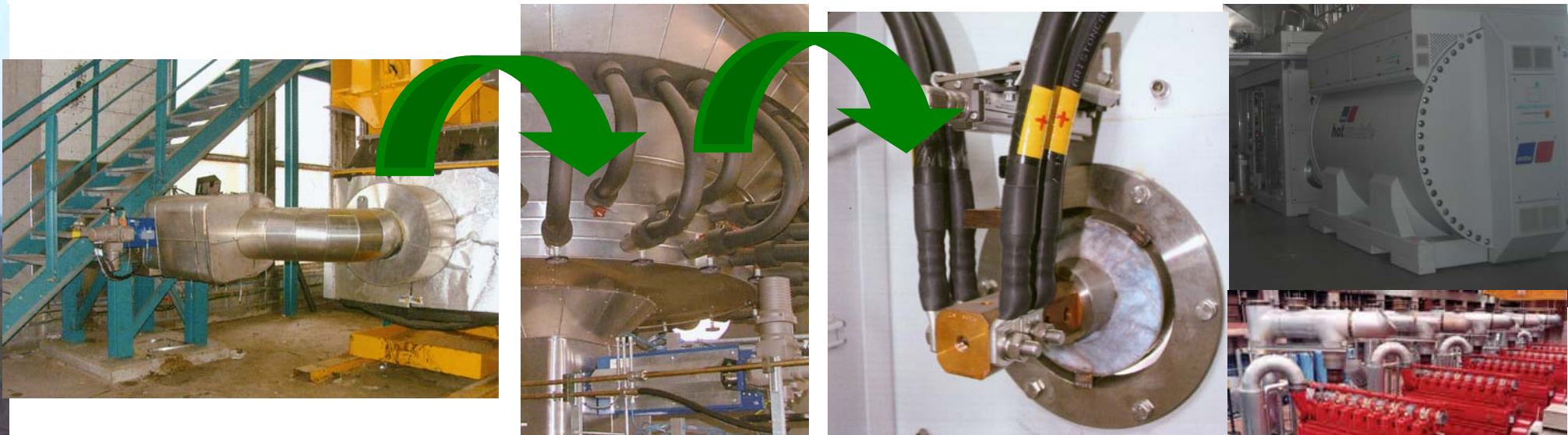
Feeding – Crushing – Fe separation – Sieving - <40 mm into the AD reactor – AD – BG fuel cell/gas engine
