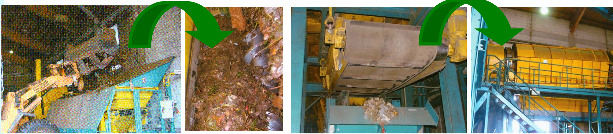
Feeding – Crushing – Fe separation – Sieving - <40 mm into the AD reactor – AD – BG fuel cell/gas engine
