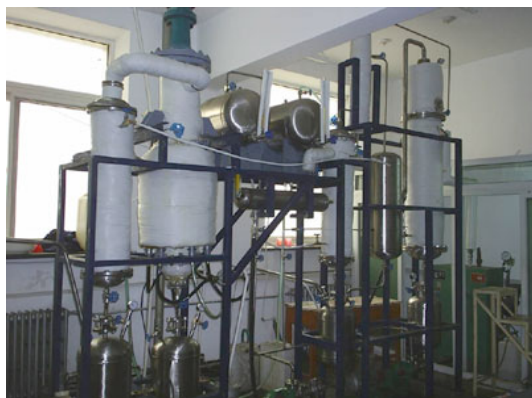
The medium test device of physic nut bio diesel with capacity of 200 tons per year
