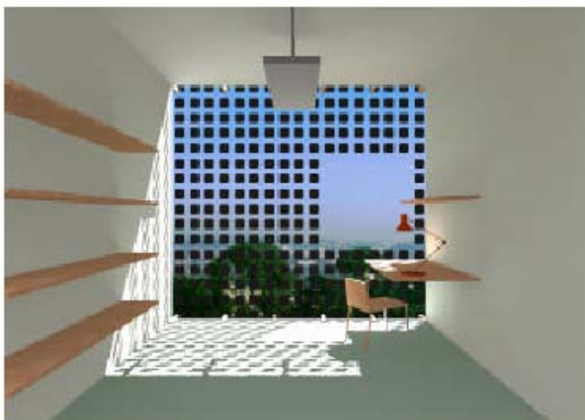
Figure 4.2.1 PV integrated with glazing (Andresen I,2002, p11)
