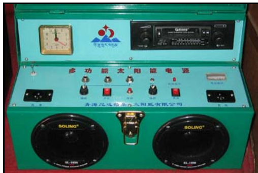
A Chinese manufactured charge controller with integrated clock and radio.
