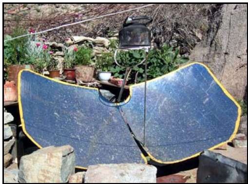
A parabolic solar water heating device used in Southwestern China.
